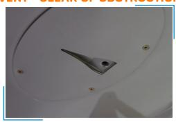
Each TKS fluid tank is vented through a NACA-style duct on the bottom of the wing, just outboard of the tank.
